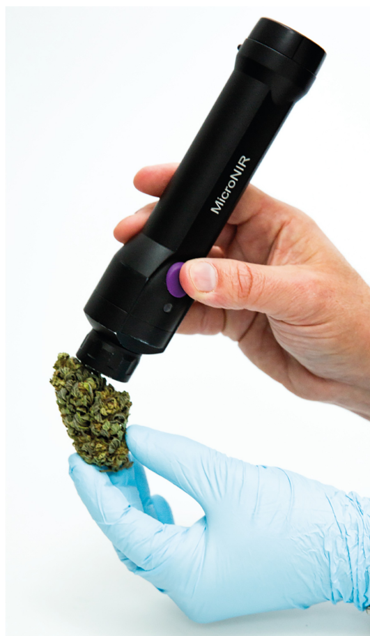
Figure 7. Illustration of the analysis of marijuana and resin cannabis specimen using the MicroNIR Onsite-W .
