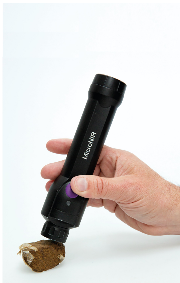
Figure 7. Illustration of the analysis of marijuana and resin cannabis specimen using the MicroNIR Onsite-W .
